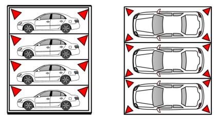
Figure 39: Sprinkler arrangement for AVPS suggested by FRV and AFAC. Reproduced from [16], [30].
