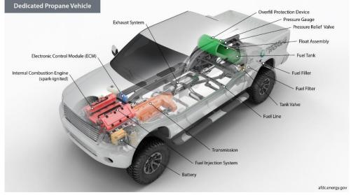
Figure 32: Typical liquified petroleum gas (LPG) vehicle layout. © Alternative Fuels Data Center.
