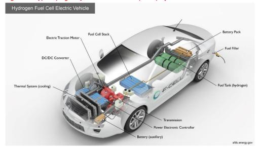
Figure 31: Typical hydrogen fuel cell electric vehicle (HFCEV) layout. © Alternative Fuels Data Center.
