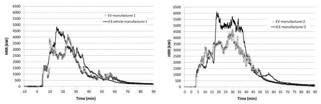
Figure 33: Comparison of the HRR from EV and ICEV tests from two manufacturers. Reproduced from [155].
