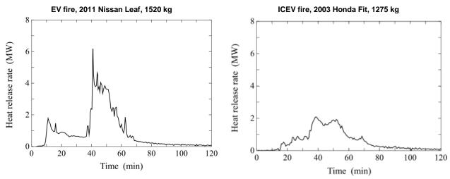
Figure 34: Comparison of the HRR from EV and ICEV tests from two manufacturers. Reproduced from [156].
