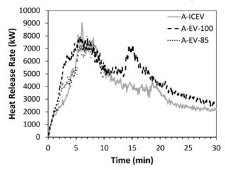
Figure 35: Comparison of the HRR from an EV at 100% and 85% charge, and an ICEV. Reproduced from [158].
