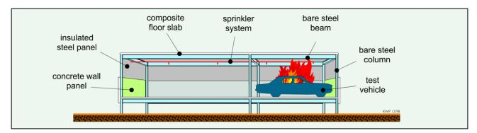
Figure 8: Isometric section drawing showing closed carpark experiment arrangement. Reproduced from [49]. © BHP.
