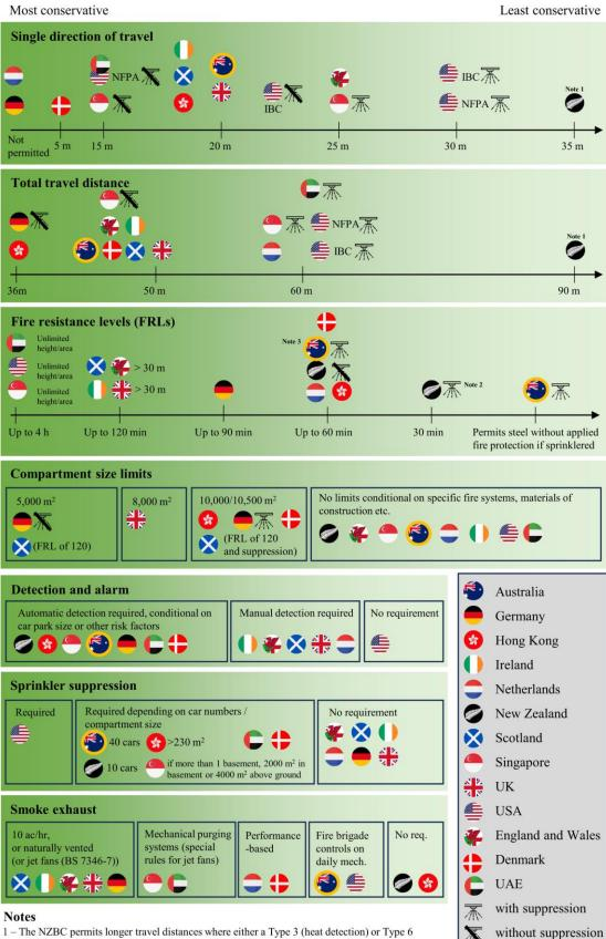
(sprinkler) system is installed (45 m / 110 m or 70 m / 180 m single / total travel distances for Type 3 and Type 6 systems respectively).
