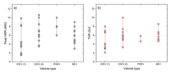
Figure 37: a) Peak HRR and b) Total Heat Released for ICEVs, PHEVs and BEVs. 'ICEV (1)' represents vehicles manufactured before 2000, whereas 'ICEV (2)' represents vehicles manufactures after 2000. Reproduced from [160].
