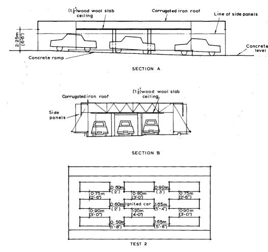
Figure 4: Section and plan views of the UK JFRO carpark experiments. Reproduced from [35].
