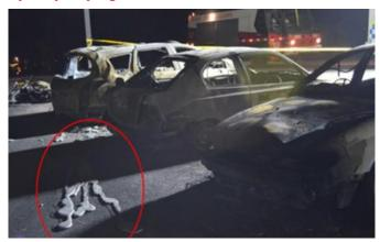
Figure 16: Molten aluminium from one of the cars involved in the Sydney Aquatic carpark fire. Reproduced from [70].
