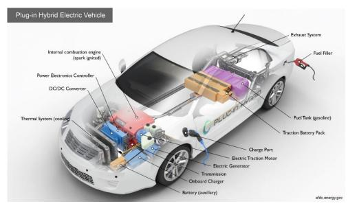
Figure 30: Typical plug-in hybrid electric vehicle (PHEV) layout. © Alternative Fuels Data Center.
