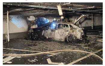
Figure 18: EV burnt out after the fire. Reproduced from [73].
