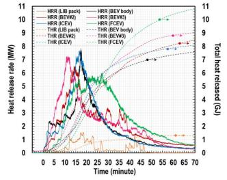
Figure 36: Comparison of the HRR from a BEV, ICEV and Hydrogen FCEV. Reproduced from [159].
