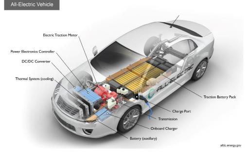
Figure 28: Typical battery electric vehicle (BEV) layout. Alternative Fuels Data Center.
