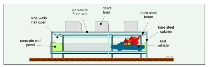
Figure 5: Isometric section drawing showing open-deck carpark experiment arrangement. Reproduced from [49]. © BHP.
