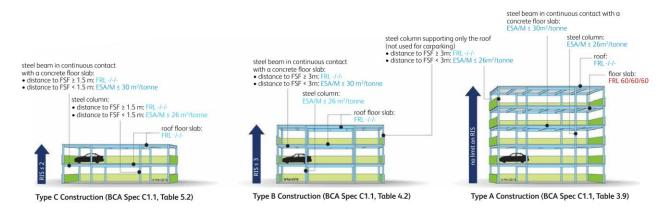
Figure 1: Structural FRL requirements for carparks within the NCC 2019. Reproduced from [6]. © Liberty Steel.
