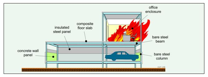
Figure 12: Isometric section drawing showing experiment arrangement with fire originating in another part of the building. Reproduced from [49]. © BHP.
