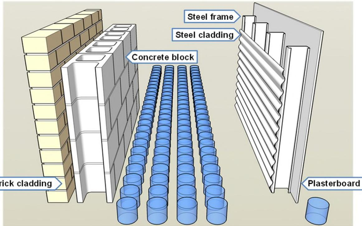
Relying on the hygric capacity of the building envelope construction is not a panacea for avoiding problems with water vapour. Some of the capacity will be needed to deal with periodic wetting by rain, surface water or rising groundwater, and some for construction moisture in the building fabric itself (e.g. water in concrete slabs or steam cured concrete blocks).
