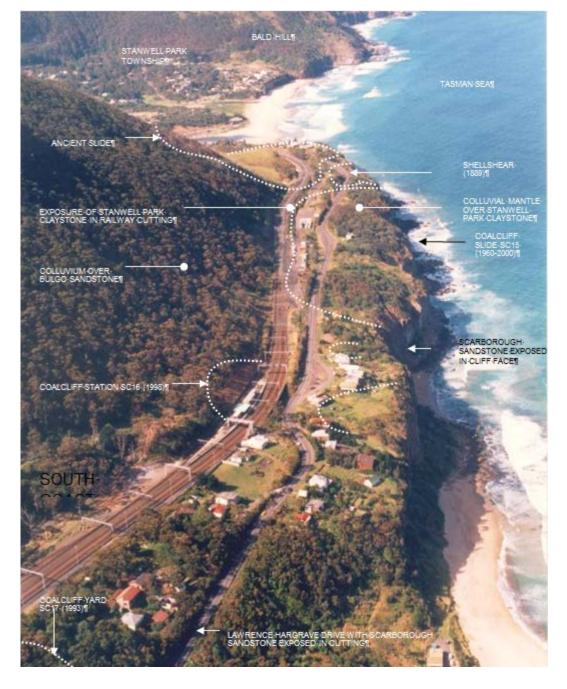
Figure 7 – Geological setting of recurring landslide events (Photograph courtesy of Phil Flentje)
