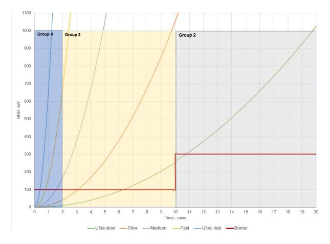
Figure 1 Plot of T-Squared Fires, ISO 9705 Burner Heat Release Rate and AS 5637 Group Number Classifications
