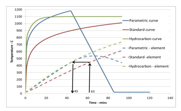
Figure 3 Conversion of Fire Resistance Period to Fire Scenario Time
