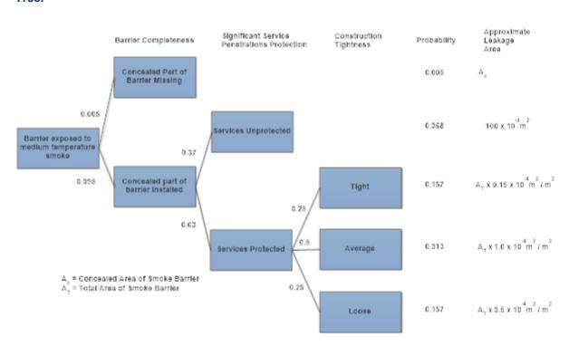
Figure 1 Example Derivation of Performance Distribution for a Smoke Barrier using an Event Tree.
