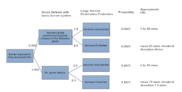
Figure 2 Example Derivation of Performance Distribution for a Smoke Barrier using an Event Tree.
