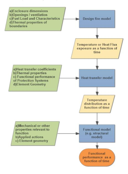
This Data Sheet relates to the *design fire* model stage which derives the enclosure conditions which can then be used as an input for subsequent analysis of the functional performance of an element, service or part or all of a structure.
