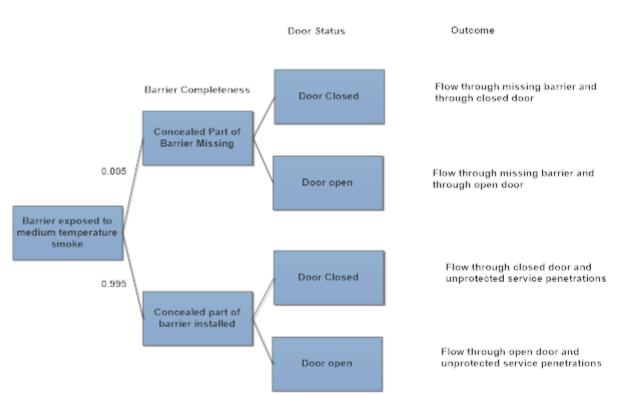
Figure 2 Example Derivation of a Performance Distribution for a Smoke Barrier Using an Event Tree
