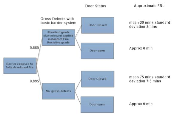
Notes Probabilities of door open case will depend on the application. Approximate FRLs for door closed cases may require modification if FRL distribution for doors is lower than the base wall. Further Guidance is provided in Data sheet C7
