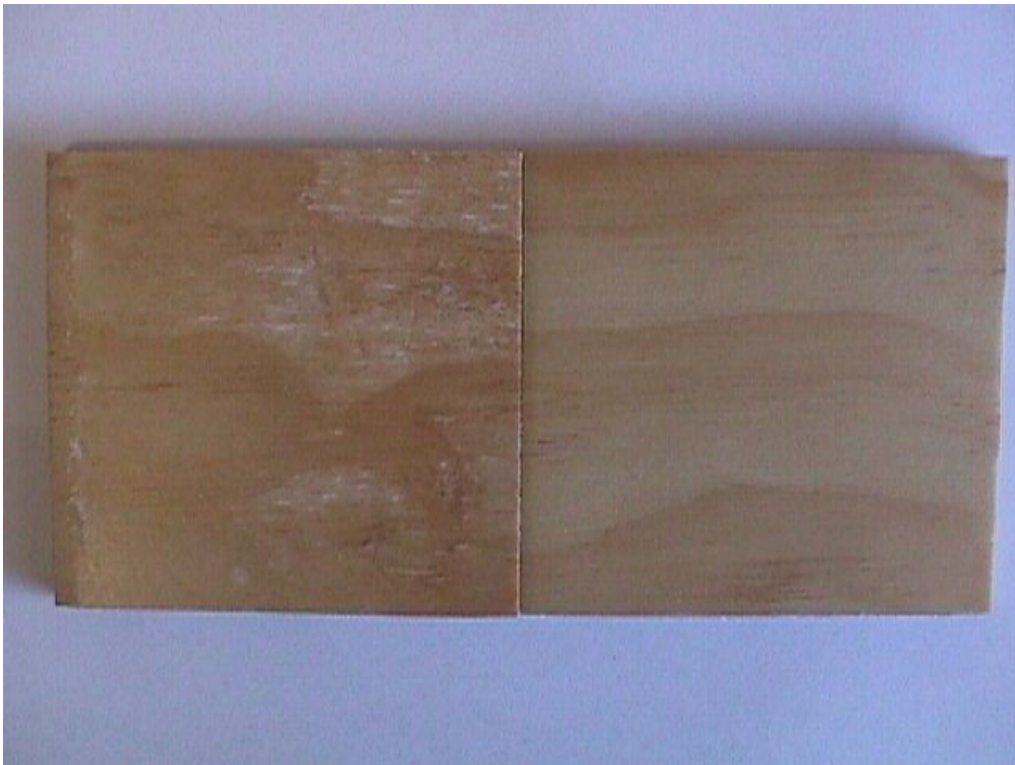
Figure 2: Plywood Samples Coated with a Clear Intumescent System, After Washing Process W2 (left) and Unweathered Sample (right)
